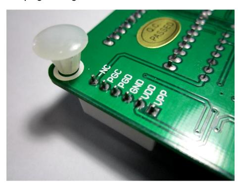
Just connect this pins with the equivalent in the PIC and program by the same way .
