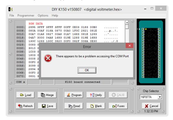
so you have type a wrong COM Port or didn't install the driver correctly
